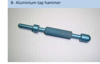
The B- Aluminium tap hammer, is used to detect delamination (separation of plies) and dis-bonds from the core in advanced composite structures.
