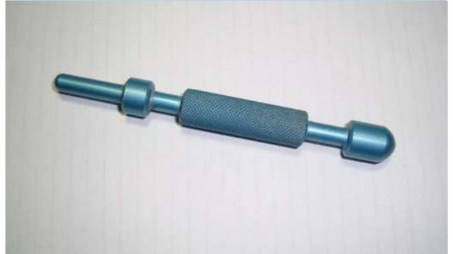
The B- Aluminium tap hammer, is used to detect delamination (separation of plies) and dis-bonds from the core in advanced composite structures.
